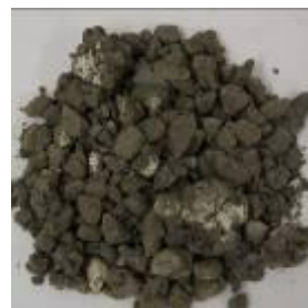
High Damage (100% particle loss)
