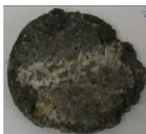
Low/Moderate Damage (35% particle loss)
