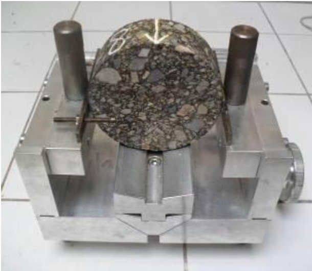
Photo 9: Gluing rack designed by VTI, a requisite for proper bonding on diametral plane.
