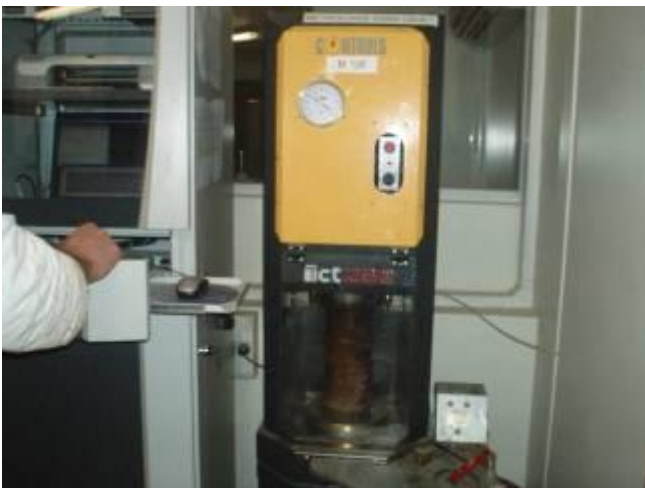
Photo 2: Gyratory Shear Press used to manufacture specimens with 100mm diameter and a predefined air void content in % (geometrical).
