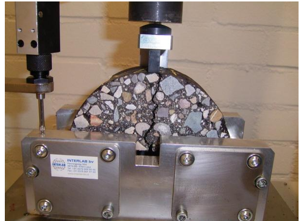
Figure 4: The SCB-test in progress
