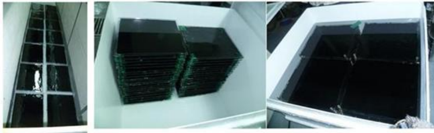
Figure 4. Asphalt binders submerged in water
