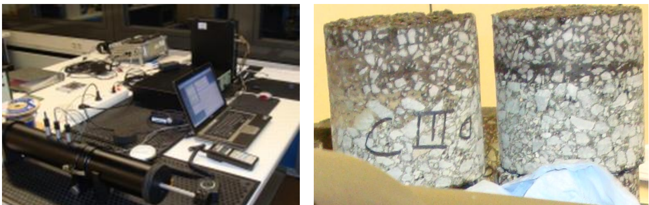
Figure 7: test methods impedance in impedance tubes (ISO 10534-2:1998)
