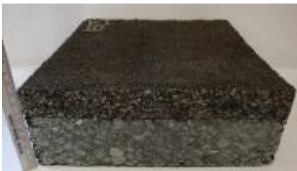
Figure 4: Composite slabs made of asphalt wearing course and asphalt binder course material
