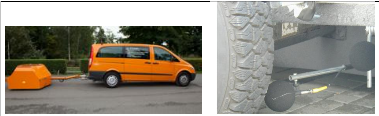
Figure 10: Close-Proximity Method (CPX-Method)
