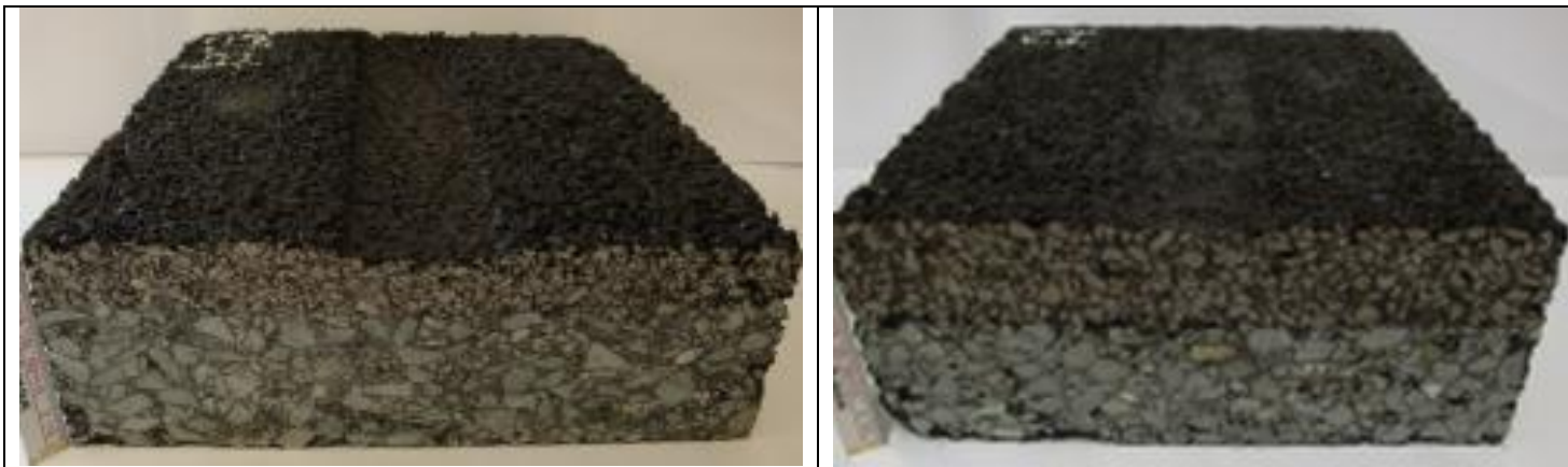
Figure 3: Composite slabs made of asphalt wearing course and asphalt binder course material (PMA und SMA)
