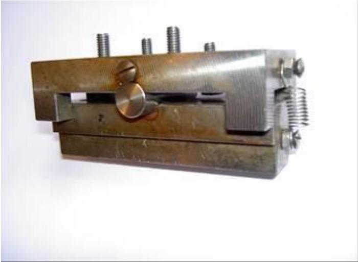
**Figure 5: Flexible upper loading strip according to EN\_12697-24\_2004**
