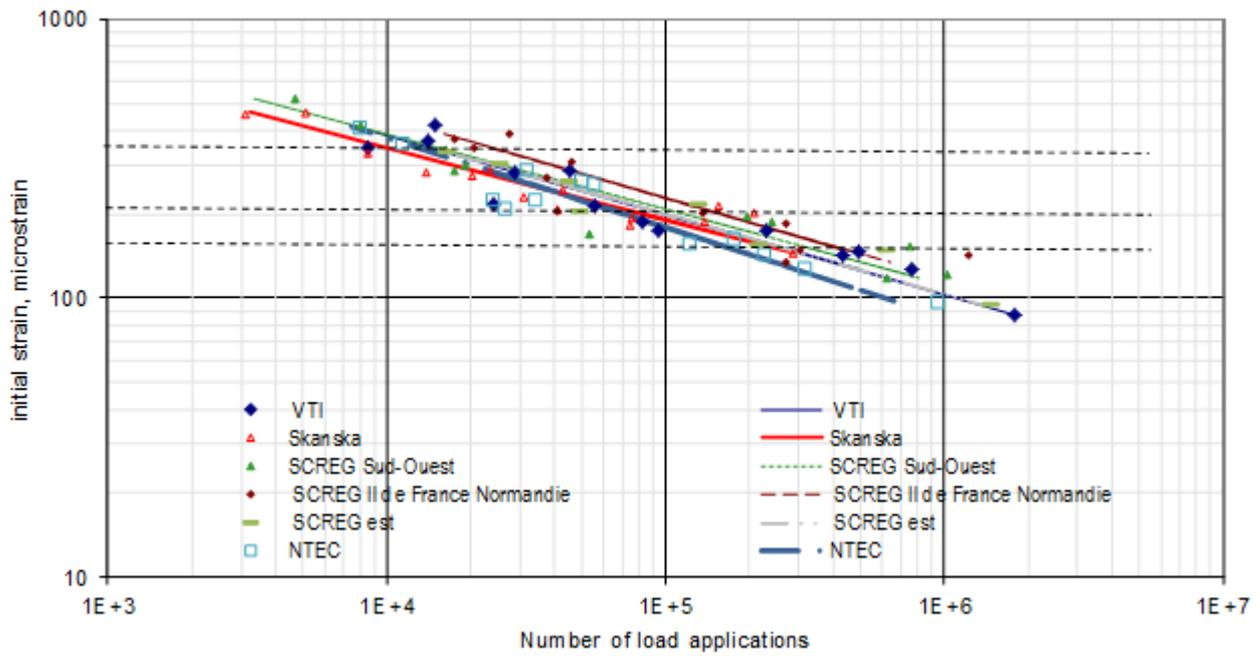
Figure 6: Fatigue relationships of asphalt mix AG16.
