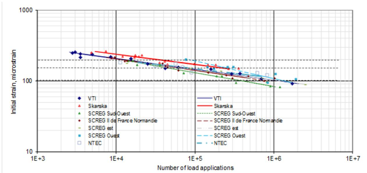
Figure 7: Fatigue relationships of asphalt mix EME14.
