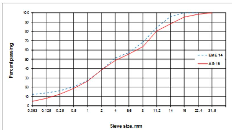
**Figure 1: Grading curves of The AG16 and EME14 mixes**
