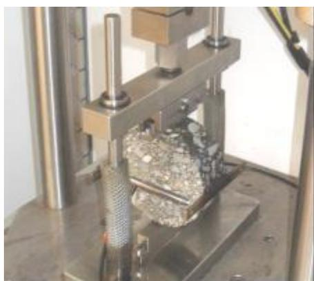
**Figure 2: Cooper NU14 used by the SCREG laboratories.**
