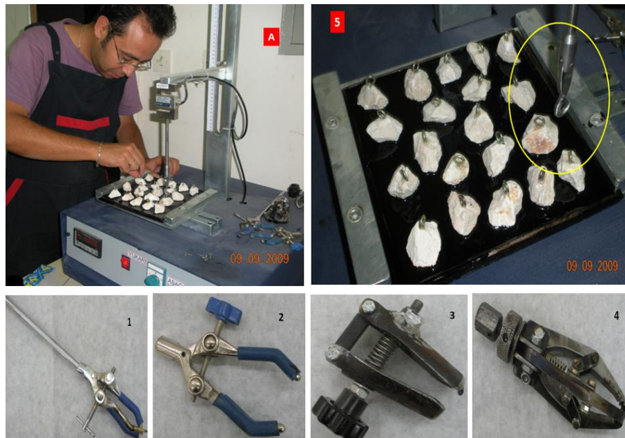
Figure 1. SDU Pull-Out Test Device (A), SDU Pull-Out Device Drilled Test Sample and hook tip (5), Different jamming tips (1-2-3-4)
