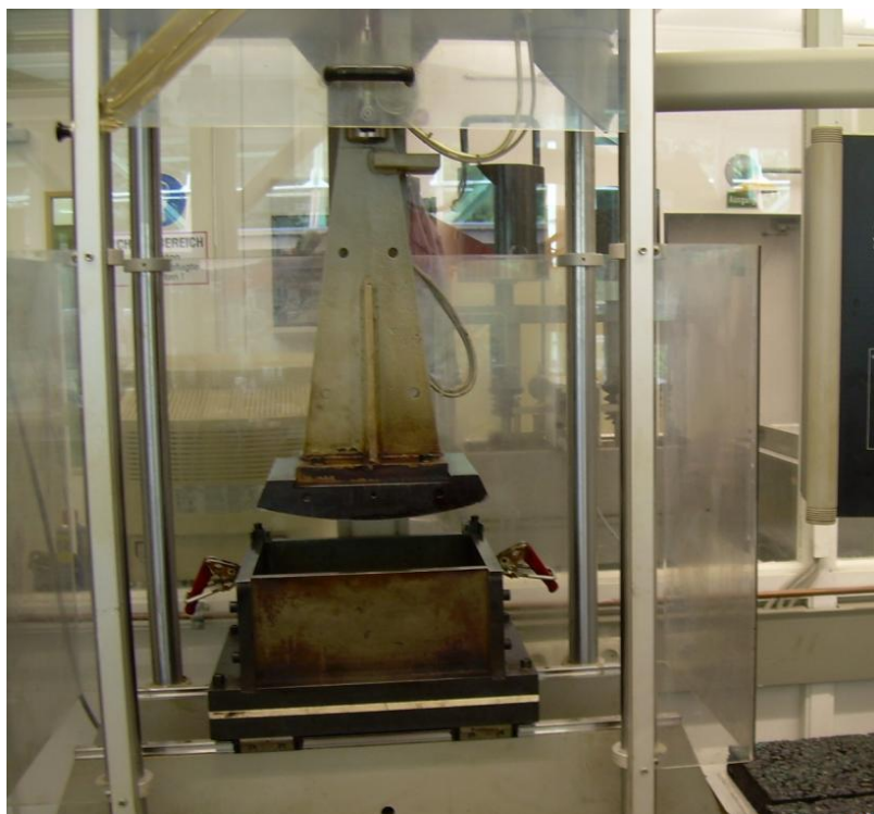
Figure 1 : Widely-used “German roller sector compactor“ for specimens 320 x 260 x max. 120 mm
