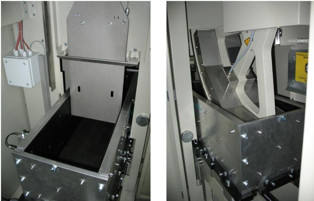
Figure 14 : Fully automated ductor (left side) and light welded roller sector with infrared heating (right side)
