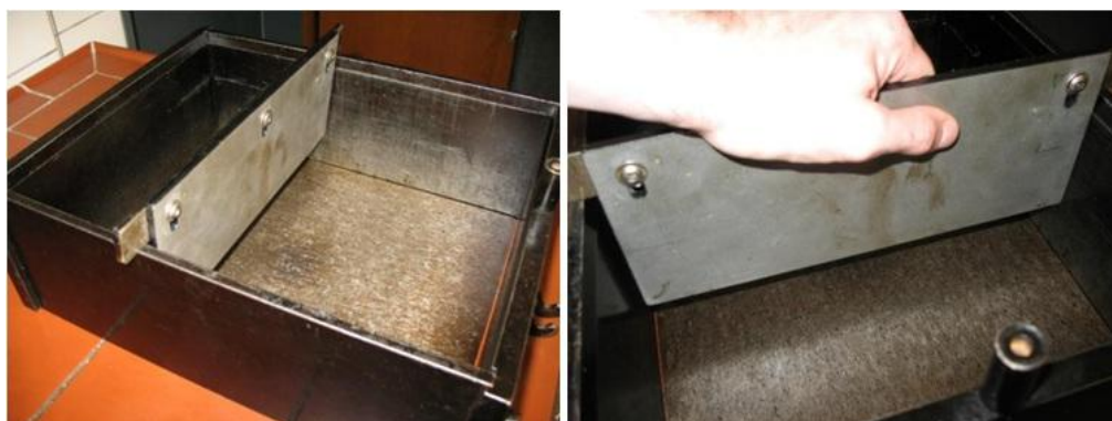
Figure 8 : Ductor (metal plate) for semi-mechanic leveling of hot mix asphalt
