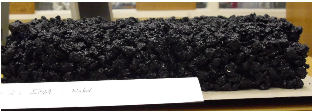
Figure 11 : Stone mastic asphalt (without compaction) with an even surface, leveled using a ductor
