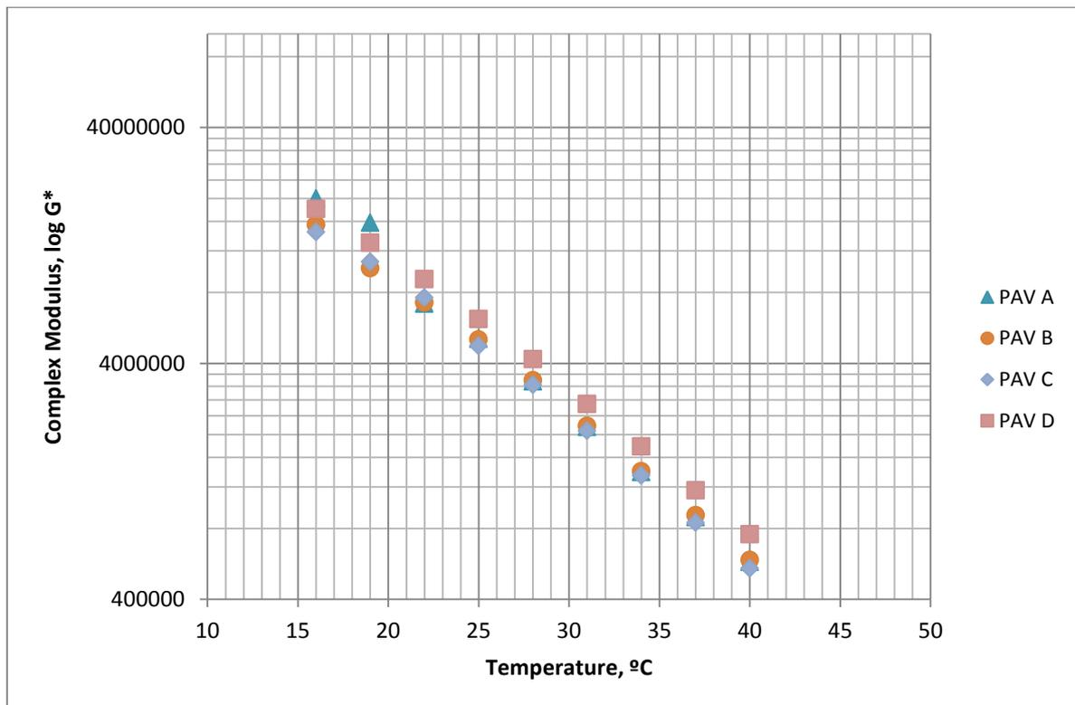
Figure 5: PAV residues, G\* vs temperature
