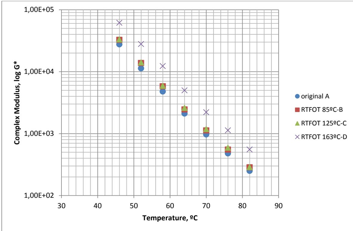
**Figure 4: RTFOT residues,  $G^*$  vs temperature**
