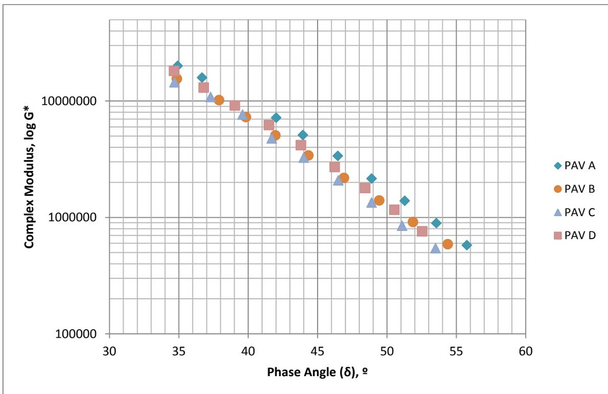
**Figure 3: Black Diagram of PAV residues**
