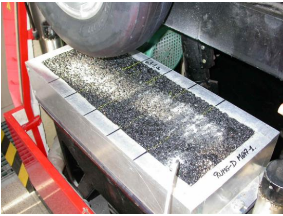
Figure 4: Wheel tracking test with wheel under angle of 5 °
