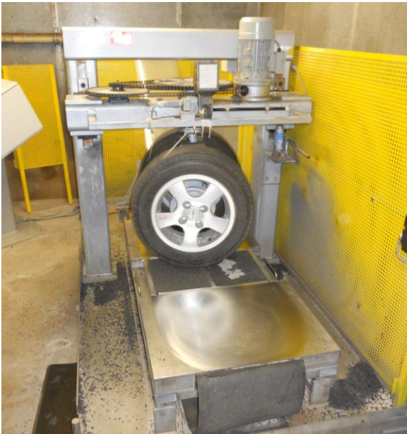
Figure 8: ARTe (test set-up at the RWTH Aachen, Germany)
