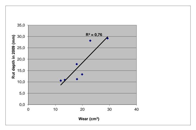
Figure 10: Correlation between rut depth measured in the field and laboratory wear (Prall test)
