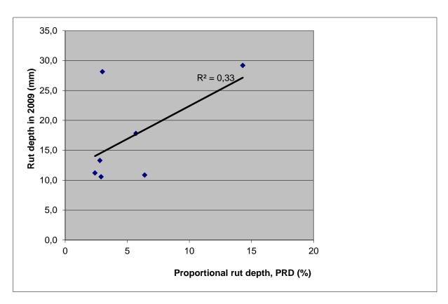
Figure 9: Correlation between rut depth measured in the field and proportional rut depth (wheel-tracking test) 5th Europitume Congress, 13-15th June 2012, Istanbul
