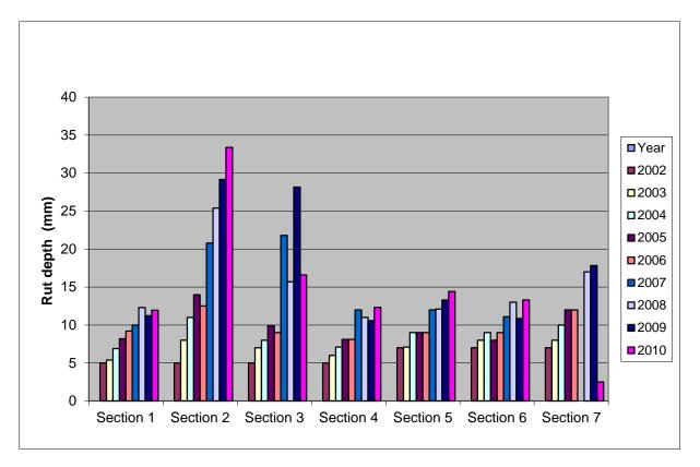
Figure 8: Measured rutting for the test sections
