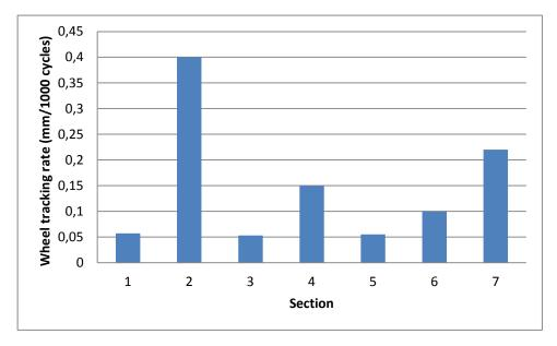
Figure 2: Results of deformation testing in the wheel track on field core samples [9].
