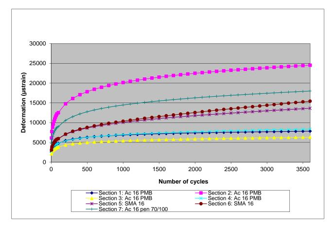
Figure 3: Results of deformation testing in NAT
