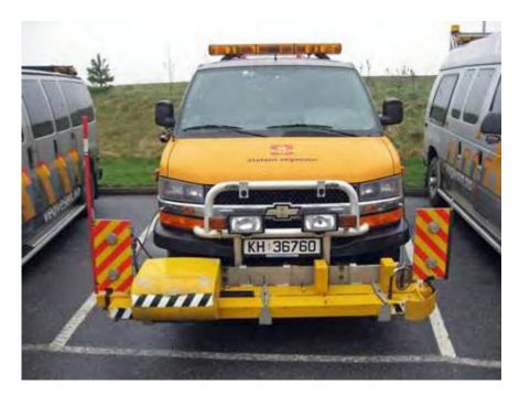
Figure 6: Ultra-sound based pavement monitoring system
