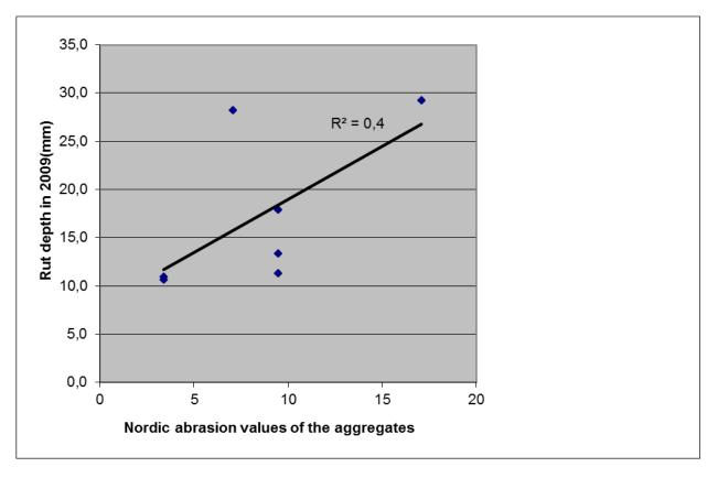
Figure 11: Correlation between rut depth measured in the field and the Nordic abrasion value of the aggregates
