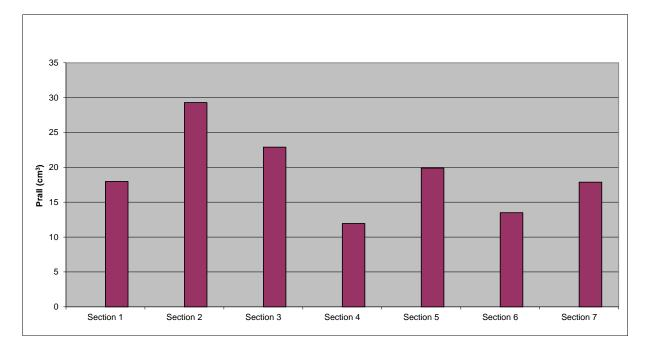
Figure 5: Results of the wear resistance test (Prall)
