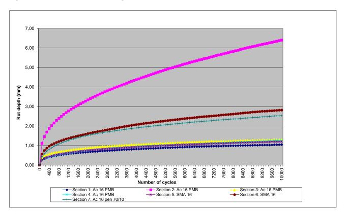
Figure 4: Results of deformation testing in the Wheel-track
