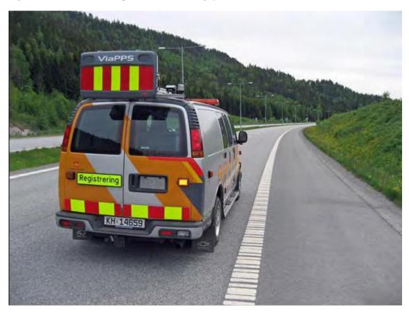
Figure 7: Pavement profile scanner (Via PPS)
