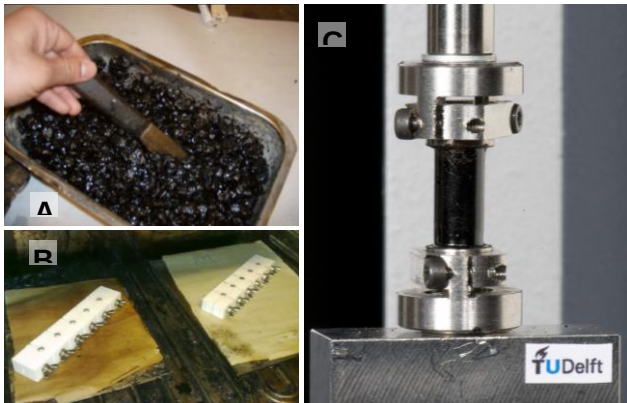
Figure 4: A: retrieving mortar from the heated mix, B: pre heating moulds in oven, C: finalized specimen in DSR ready for testing.
