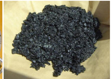
Figure 6 : Mixer [left], mixing bowl [middle], well-coated homogeneous final production at \pm 110^{\circ}\text{C} [right]
