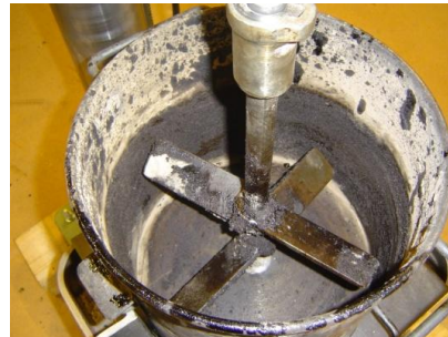
Figure 6 : Mixer [left], mixing bowl [middle], well-coated homogeneous final production at \pm 110^{\circ}\text{C} [right]
