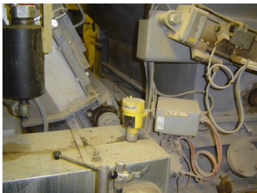
Figure 7 : Asphalt plant – Injection in parallel drum [left], foamed bitumen unit by the mixer [right]
