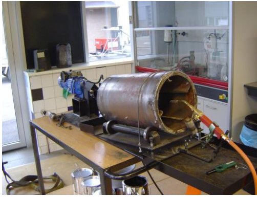
Figure 4 : Lab drying drum [left] and Foamed bitumen installation at the final mixer [right]
