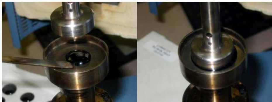
Figure 1: Tribo-Rheometry testing fixture and sample loading
