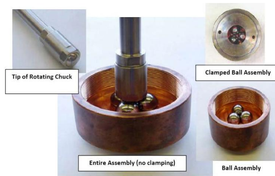
Figure 3: Asphalt Lubricity testing fixture (from Hanz, et al. [9])
