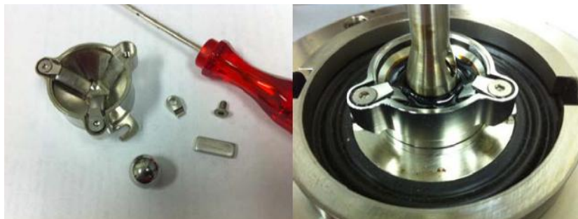
Figure 5: Cup and Plated assembly for the Tribology fixture.
