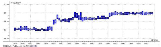
Figure 5 - Predictions and standard deviations for CO2 (fuel natural gas)
