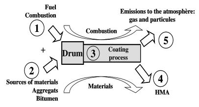
of control [4]. Among the out of control fluctuations, we can mention the moisture of the aggregates, which is entirely dependent on the storage and the meteorology, and the fuel variations (public network). However, even the parameters considered as a priori under control are subject to the variations resulting from the needs of the road construction site [5]. It is the case of production rate, input materials regularity and HMA temperature.
