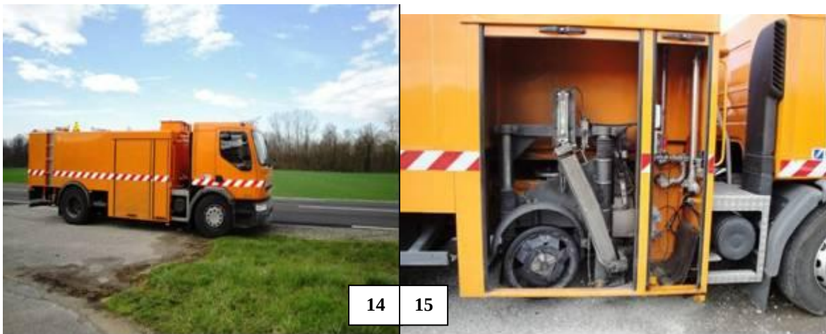
Figure 14: Sideway Force Coefficient Routine Investigation Machine for the CFT measurement. Figure 15: Device for measuring (wheel and water injection)
