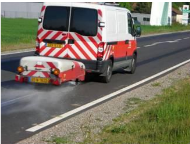
Figure 16: Device ADHERA for measuring the Sideways Force Coefficient (C.F.L.) on the pavement.
