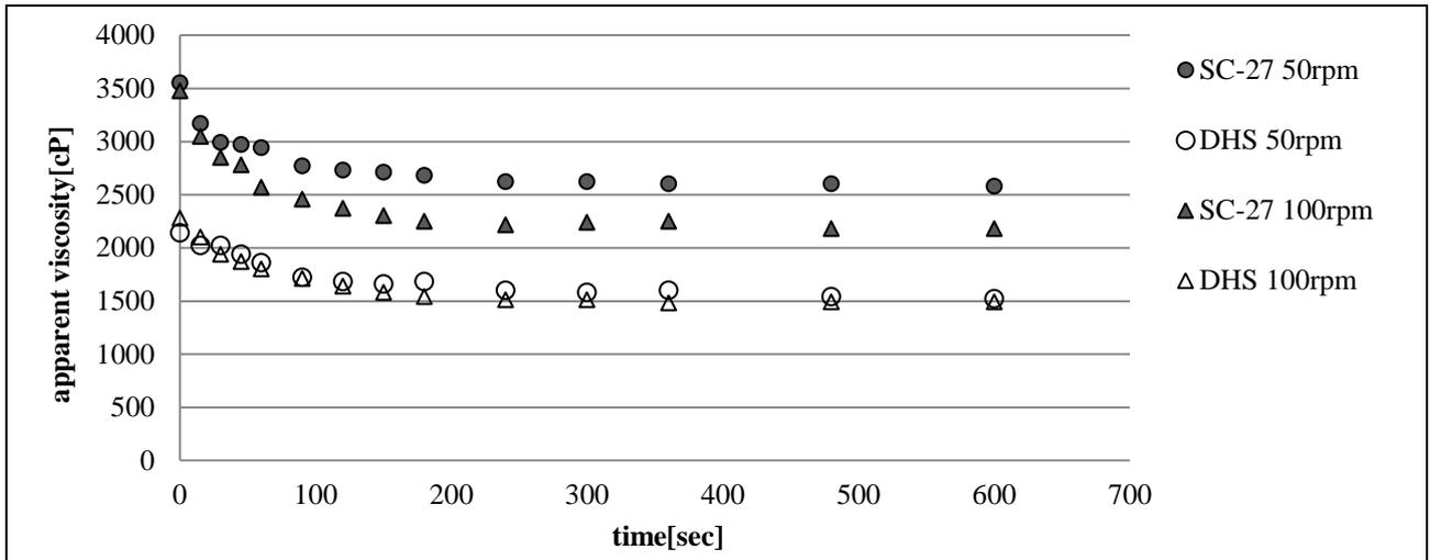
**Fig. 8 Apparent viscosity of a TR-MB at 177.5°C by using HA viscometer at 50 – 100 RPM**
