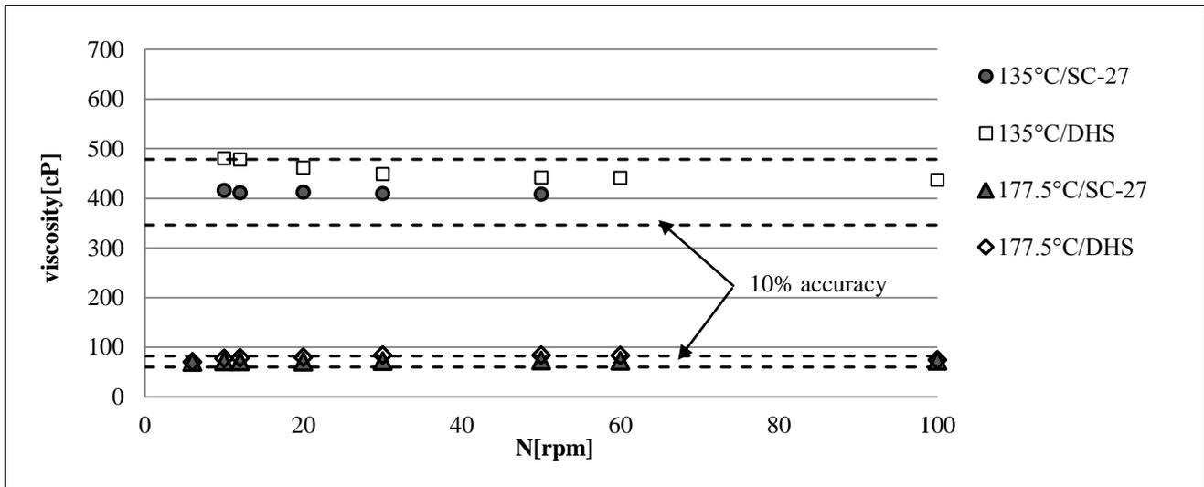
Fig. 6 Viscosity measurements by using LV on a 40/60 pen bitumen at T=135°C and 177.5°C
