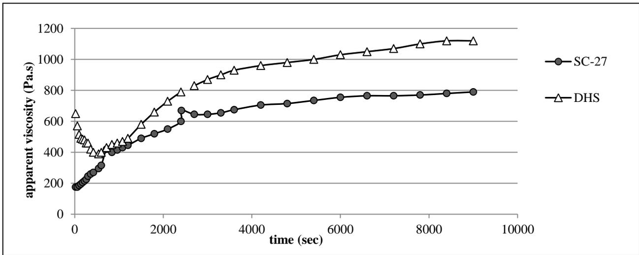
**Fig. 9 Results of constant monitoring using the Brookfield Viscometer as a low shear mixer at 177.5°C**
