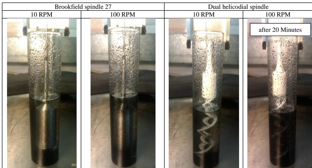
**Fig 2. Preliminary study: after 15-20 minutes mixing**
