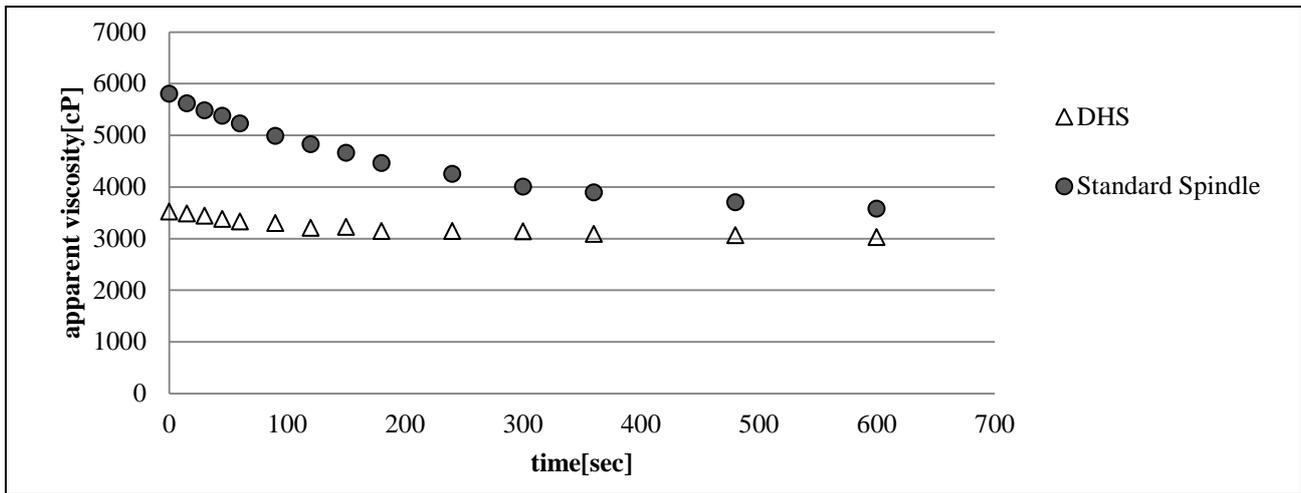
**Fig. 7 Apparent viscosity of a TR-MB at 177.5°C by using LV viscometer at 12 RPM**
