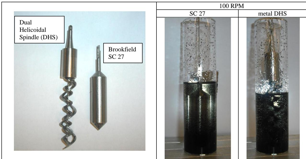
**Fig. 3. Steel DHS and its effect of keeping particles suspended after 15-20 minutes of mixing**
