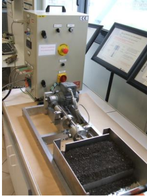
Picture 1: Nynas workability measurement tool
