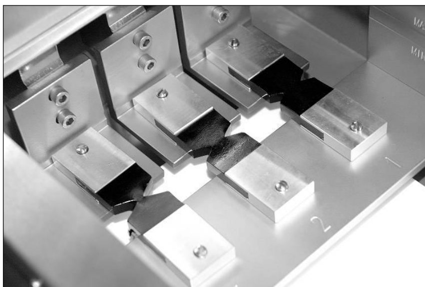
Figure 2 – Double-edge-notched tension (DENT) specimens just prior to conditioning and testing. Note: Ligament lengths shown are (1) 15 mm, (2) 10 mm, and (3) 5 mm.
