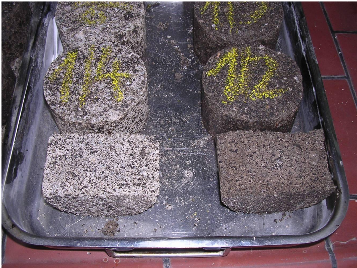
Figure 1: Appearance of the foam bitumen stabilised material specimens – dry (left) and soaked (right)
