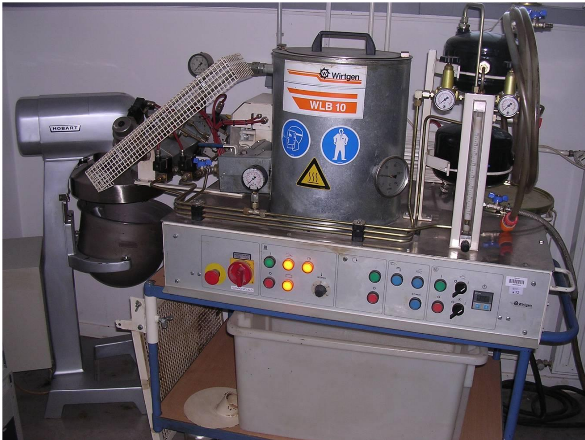
Figure 3: Laboratory equipment for foamed bitumen stabilised material mixing
