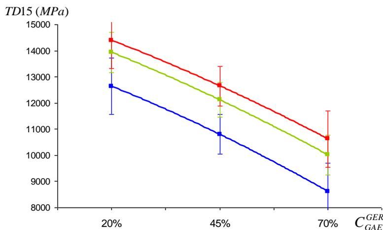
**Fig. 7: Direct tension modulus at 15°C as a function of recycling rate for a mixing time of 40 s (110°C in blue, 135°C in green, 160°C in red)**
