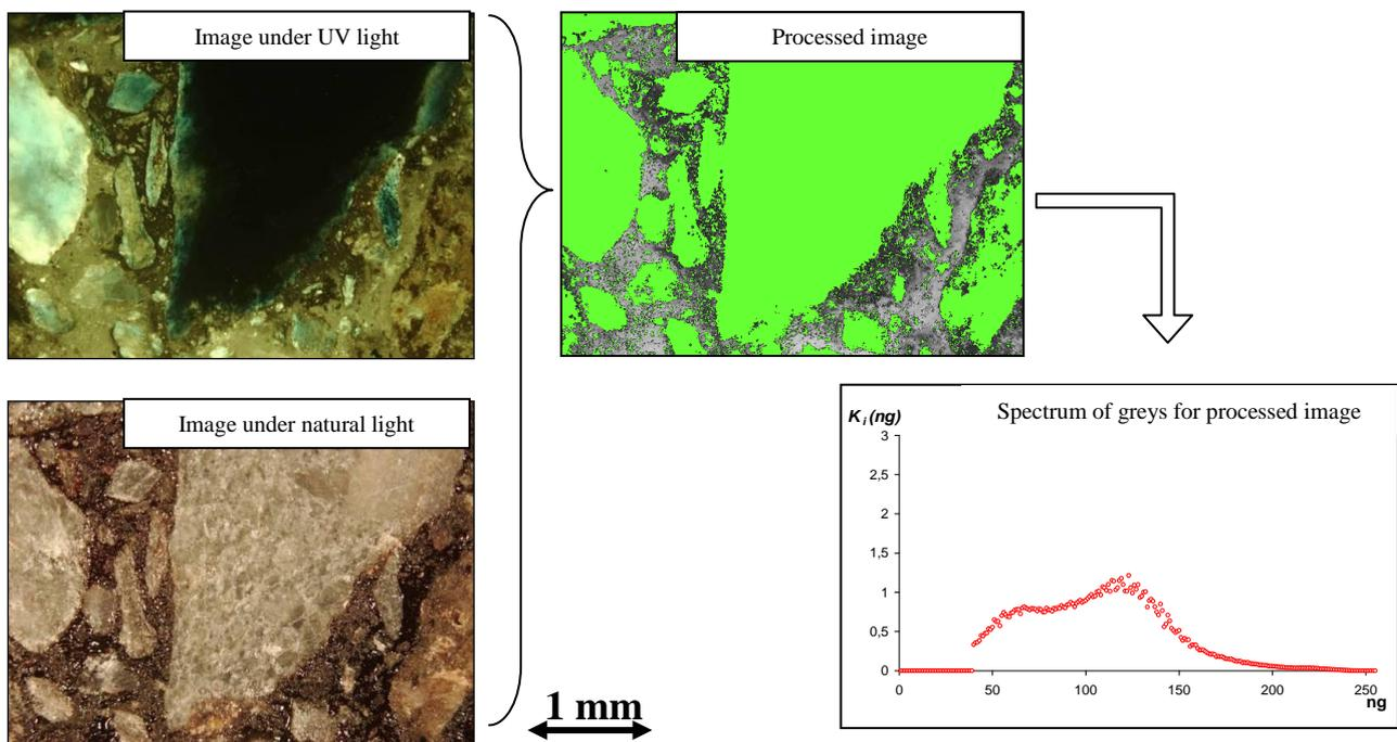
**Fig. 2: Principle of process to determine distribution of RAP binder in the recycled asphalt concrete**
