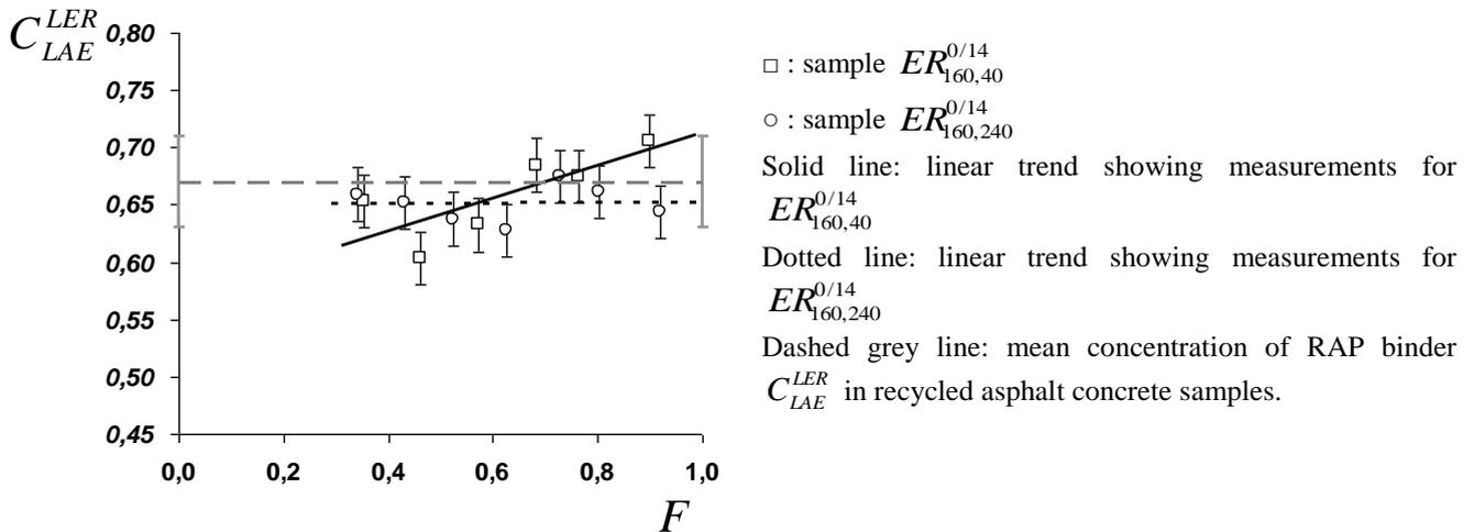
**Fig. 12: Graph showing results from data analysis of lixiviation of recycled asphalt concrete samples produced at 160°C (samples  $ER_{160,40}^{0/14}$  and  $ER_{160,240}^{0/14}$ ) showing the evolution in concentration  $C_{LAE}^{LER}$  of RAP binder in the extracted binder as a function of mass fraction  $F$  of extracted binder**
