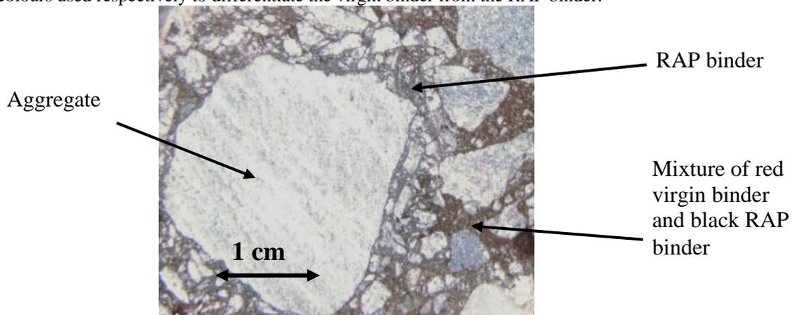
**Fig. 1: Cluster of centimetric sized reclaimed asphalt pavement at the surface of the aggregates, highlighted by the addition of binder with iron oxide pigment (red)**
