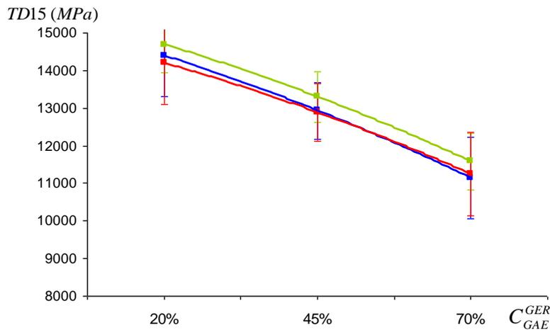
**Fig. 8: Direct tension modulus at 15°C as a function of recycling rate for a mixing time of 240 s (110°C in blue, 135°C in green, 160°C in red)**
