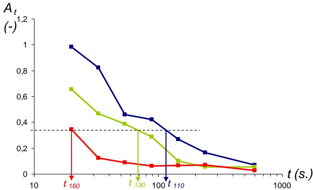
**Fig. 3: Kinetics of the disappearance of RAP clusters as a function of mixing time and production temperature (110°C in blue, 130°C in green and 160°C in red)**
