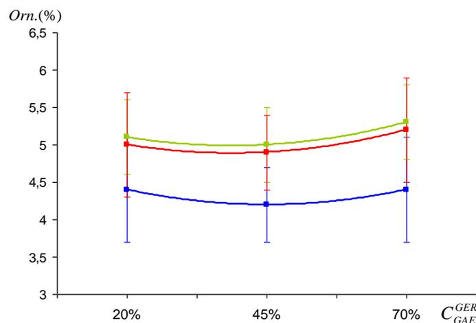
Fig. 5: Rutting as a function of recycling rate for a mixing time of 40 s (110°C in blue, 135°C in green, 160°C in red)
