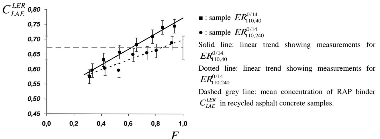
**Fig. 13: Graph showing results from data analysis of lixiviation of recycled asphalt concrete samples produced at 110°C (samples  $ER_{110,40}^{0/14}$  and  $ER_{110,240}^{0/14}$ ) showing the evolution in concentration  $C_{LAE}^{LER}$  of RAP binder in the extracted binder as a function of mass fraction  $F$  of extracted binder**
