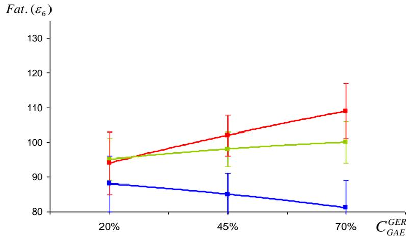
**Fig. 9: Fatigue resistance at 10°C as a function of recycling rate for a mixing time of 40 s (110°C in blue, 135°C in green, 160°C in red)**
