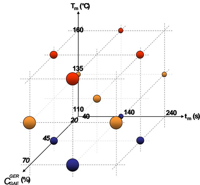
Fig. 4: Experimental points of the BOX-BEHNKEN design
