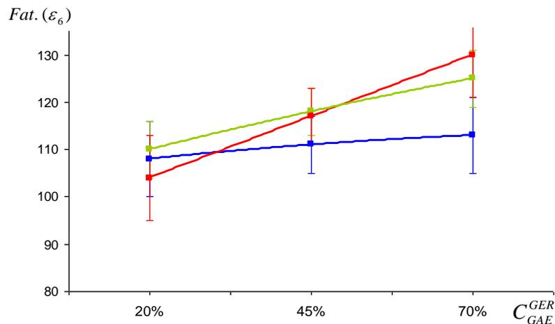
**Fig. 10: Fatigue resistance at 10°C as a function of recycling rate for a mixing time of 240 s (110°C in blue, 135°C in green, 160°C in red)**
