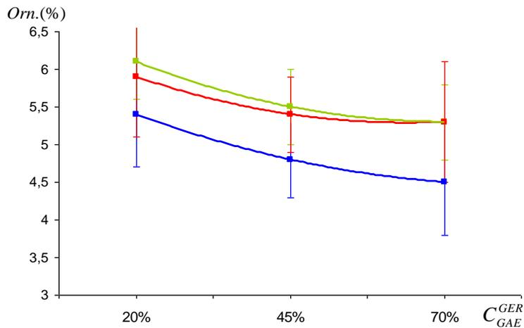
**Fig. 6: Rutting as a function of recycling rate for a mixing time of 240 s (110°C in blue, 135°C in green, 160°C in red)**
