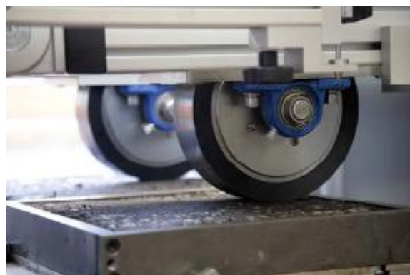
Figure 4: Test equipment for wheel tracking test
