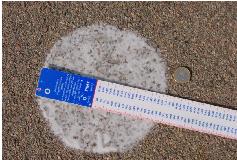
Figure 5 : Sand patch test – Macrotexture value (mm)
