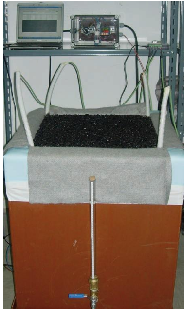
Figure 7 –Laboratory thermal energy storage tank.
