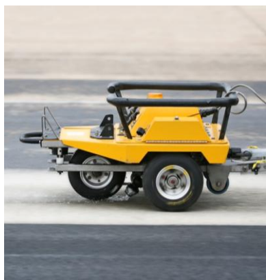
Figure 1: Low speed skid resistance measured by GripTester
