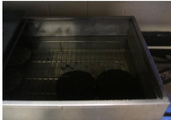
Figure 2. Submerged wet set samples in 60°C water bath
