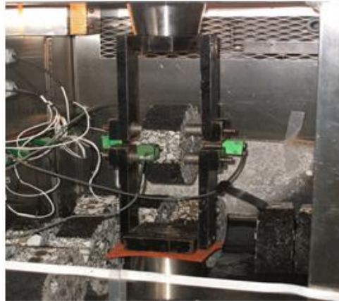
Figure 6. DCT samples placed inside fracture energy apparatus
