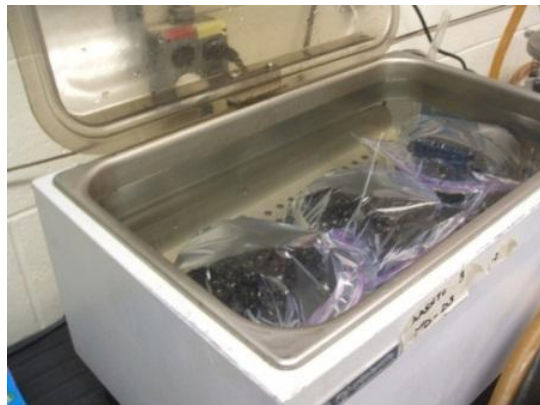
Figure 1. Wrapped AASHTO dry samples in 25°C water bath
