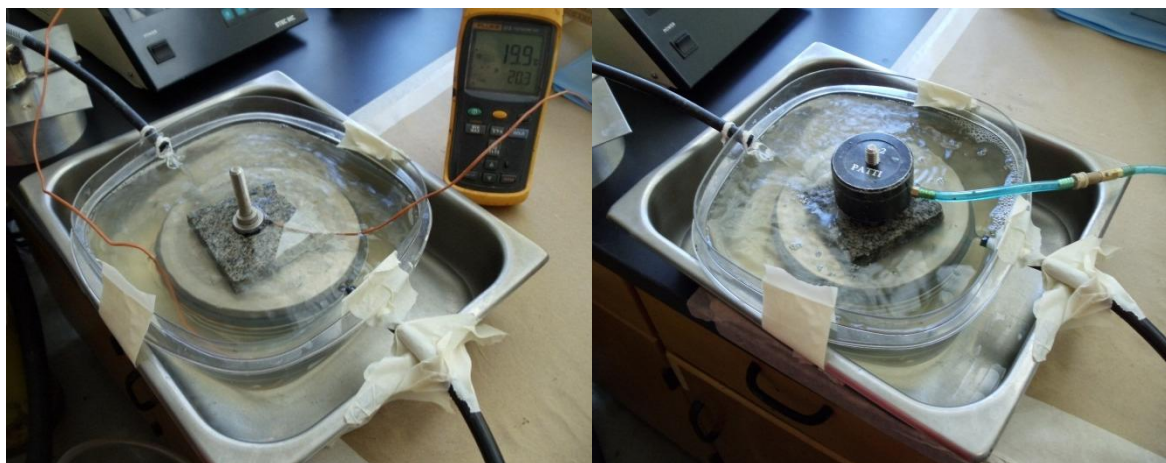
Figure 4: BBS Test With Controlled Temperature.
