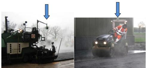
Figure 4: Laser linescanner on the paver Figure 5: GPS-equipment on a roller
