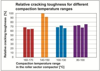
Figure 7: Relative cracking toughness for different compaction temperature ranges
