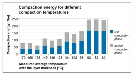
Figure 6: Compaction energy for different compaction temperatures
