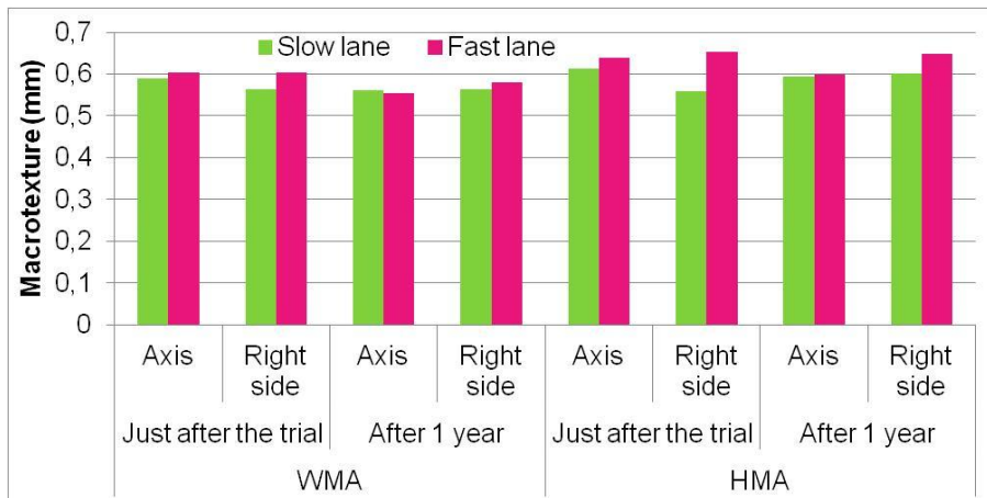
Figure 8 : Macrotexture measurements using a Rugolaser 2.
