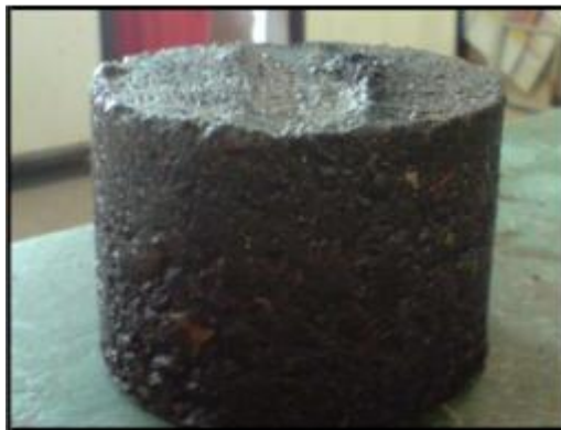
Figure 2- Waste phosphate filler sample under 6000 cycles loading
