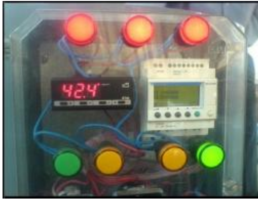
Figure 1- Cycles counter and temperature controller in wheel track machine
