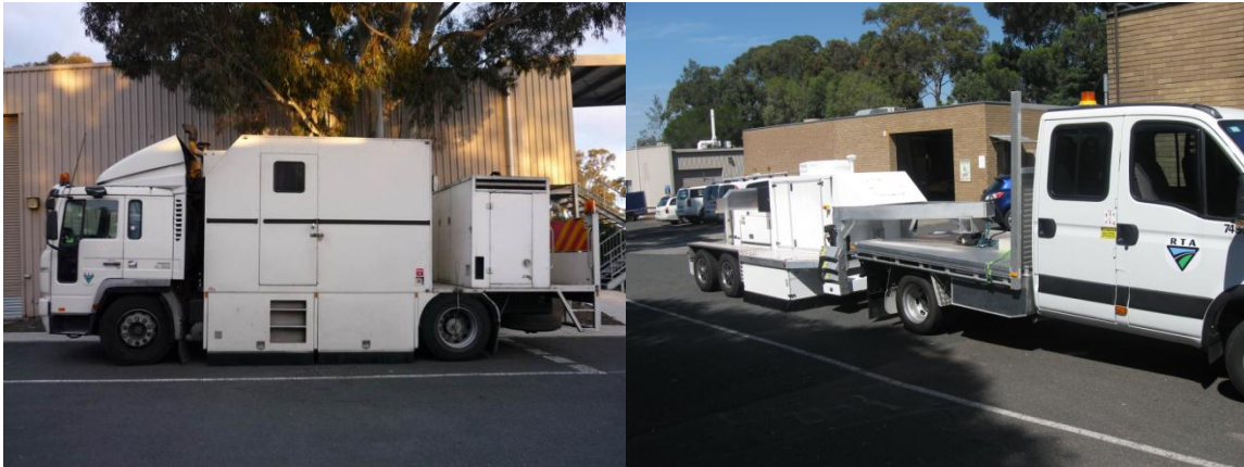
Figure 6: RoadCrack (left) and RoadCrack trailer with DLP beam in 2011
