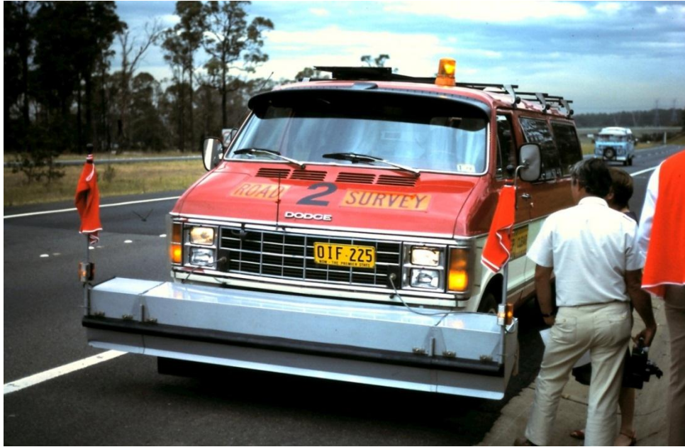
Figure 2: Swedish Laser Road Surface Tester in Australia in 1987
