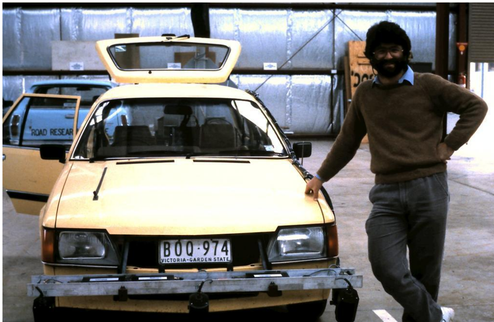
Figure 1: Original ARRB profilometer with its developer Dr. Hans Prem in August 1986
