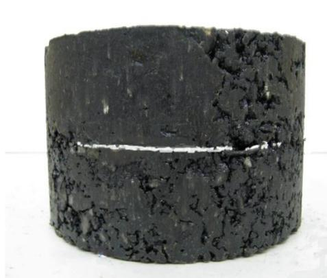
Figure 7: Series of specimens prepared for tests a) and specimen where the edge of contact surface is marked – side view b)
