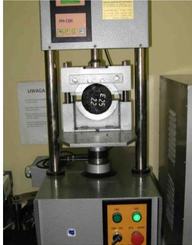
Figure 2: Monotonic shear load testing stand
