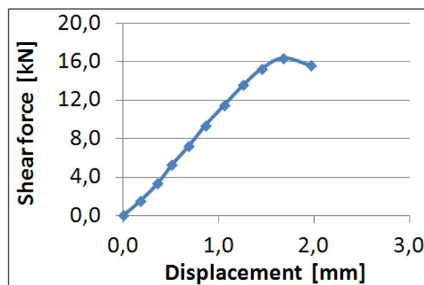
Figure 1: Shear force – displacement curve during monotonic test for a specimen of diameter 100 mm.
