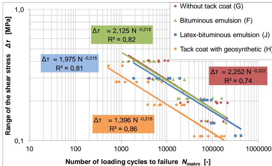
Figure 9: Wöhler fatigue curves for analysed interlayer bonding
