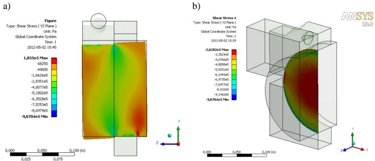
Figure 6: a) YZ shear stress distribution – side view (the symmetry plane), b) in cutting plane – front view, for shear load of 7 kN
