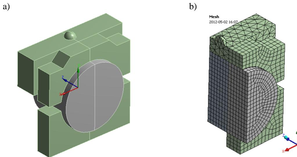
Figure 5: a) Geometric model for specimen of diameter 150 mm together with global system of coordinates XYZ, b) The mesh of the FE model with symmetry plane (elements from library of ANSYS: 20-node solid element SOLID186, 8-node contact/interface elements TARGE170 and CONTA174).
