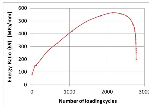
Figure 4: Energy Ratio plot during interlayer bonding fatigue test for a specimen of diameter 150 mm.
