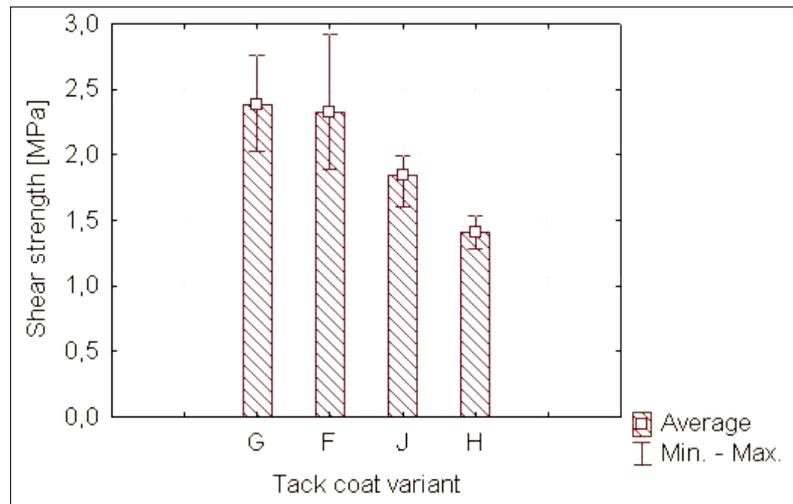
Figure 8: Average value and a min. – max. scatter for shear strength for variants of tack coat: without tack coat (G), bituminous emulsion (F), latex-bituminous emulsion (J), tack coat with geosynthetic (H).
