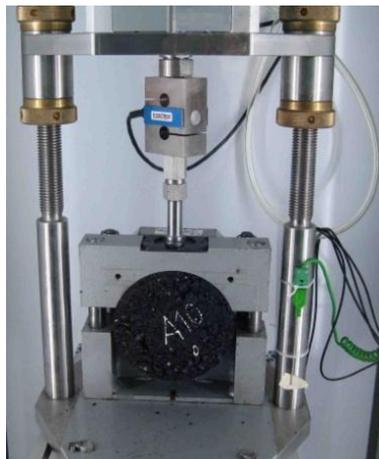
Figure 3: Fatigue testing at the shear cyclic load stand
