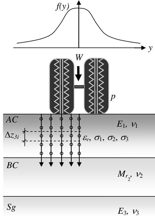
Figure 5. Schematic overview of the applied procedure to calculate the rutting. The asphalt concrete (AC) is divided into sublayers whereof the response is calculated in the middle point at desired lateral location. BC is the underlying granular base course resting on a subgrade (Sg).
