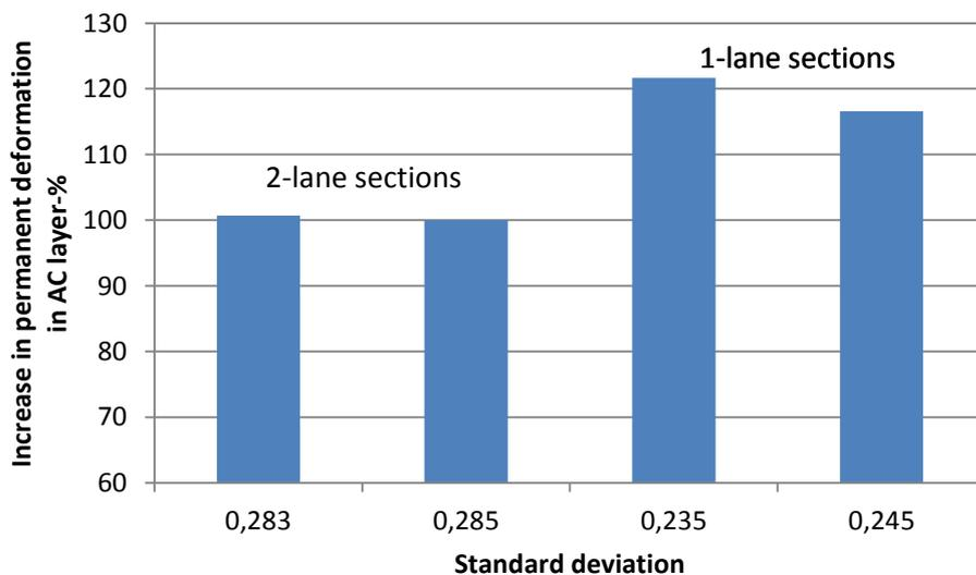
Figure 8. Increase in permanent deformation in bituminous pavement layer with respect of increase in standard deviations.
