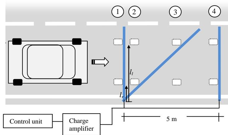
Figure 2. Schematic overview of the lateral position measuring system.
