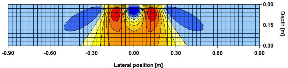
Figure 6. Distribution of the vertical permanent strain under dual wheel load (Oscarsson 2011).
