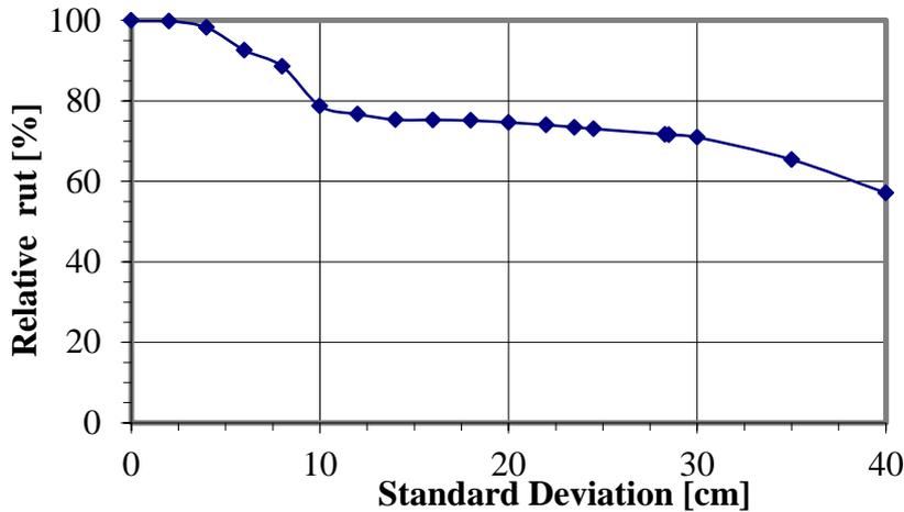
Figure 7. Relative surface rut as a function of the standard deviation of the lateral wander. The values are normalized against the maximum rut at zero standard deviation.
