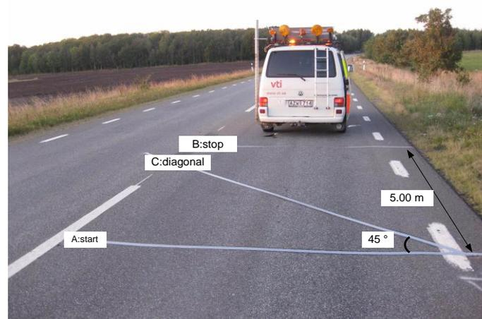
Figure 1. The setup of the system used to measure the lateral position of vehicles.
