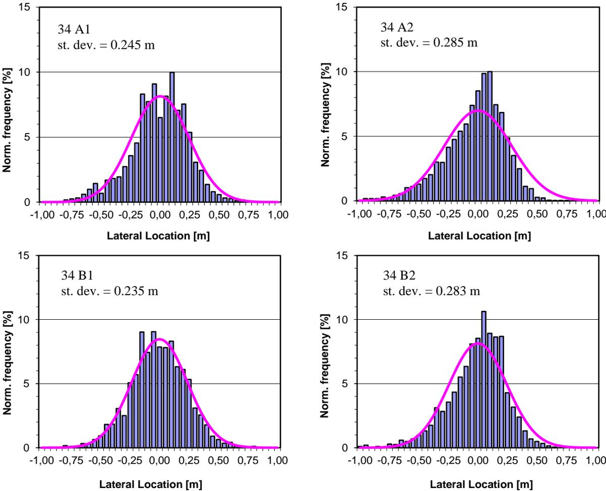
Figure 4. Normalized frequency of the lateral location of the heavy vehicles right wheel position on the arterial road Rv34 along with a normal distribution approximation. The mean value has been adjusted to zero and the standard deviation is given in the figures. A1 and B1 represent measurements on the single lane section of the road whereof the A2 and B2 are on the outer wheel lane of the two lane section.
