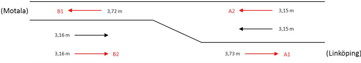
Figure 3. Lane widths and traffic directions at Road Rv34 of type 2+1 road in Southern Sweden, per each section.
