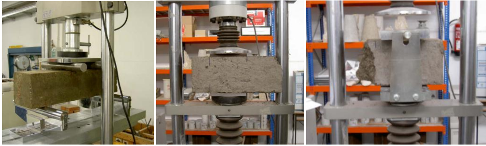
Figure 2: Bending strength trials, compressive and splitting tensile strength tests
