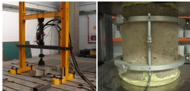
Figure 3: Dynamic and modulus of deformation test
