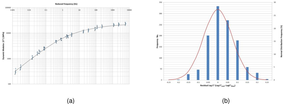
Figure 7 Typical Modulus Grouping Results and distribution of errors around the master-curve
