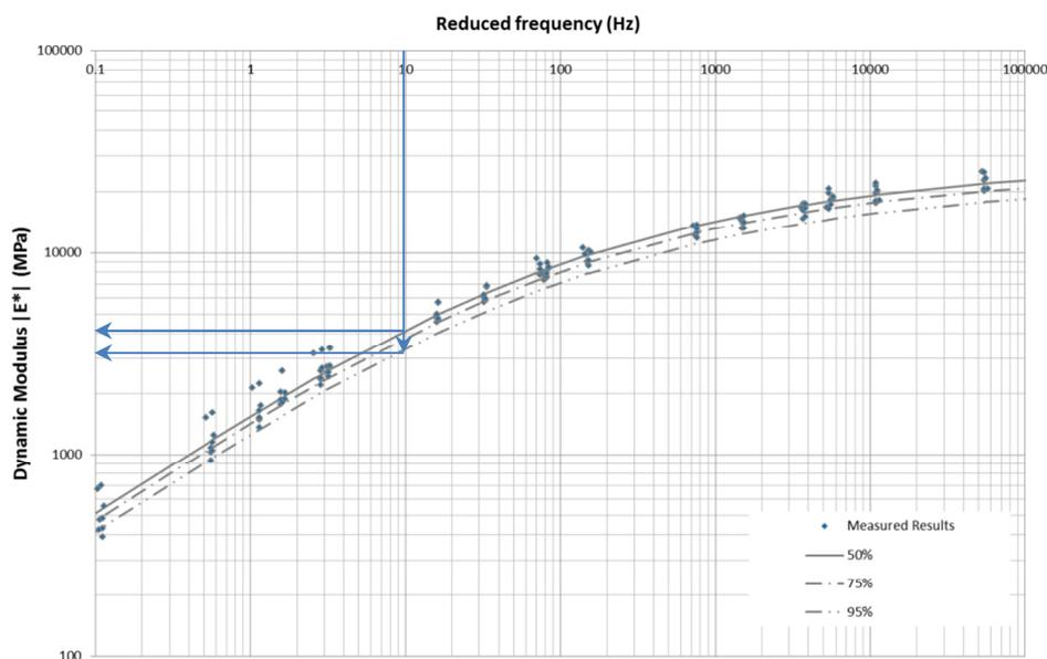
Figure 8 Confidence Interval Master-curve
