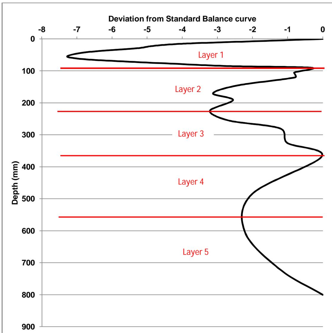
Figure 6. Normalise balanced curve with possible layers indicated
