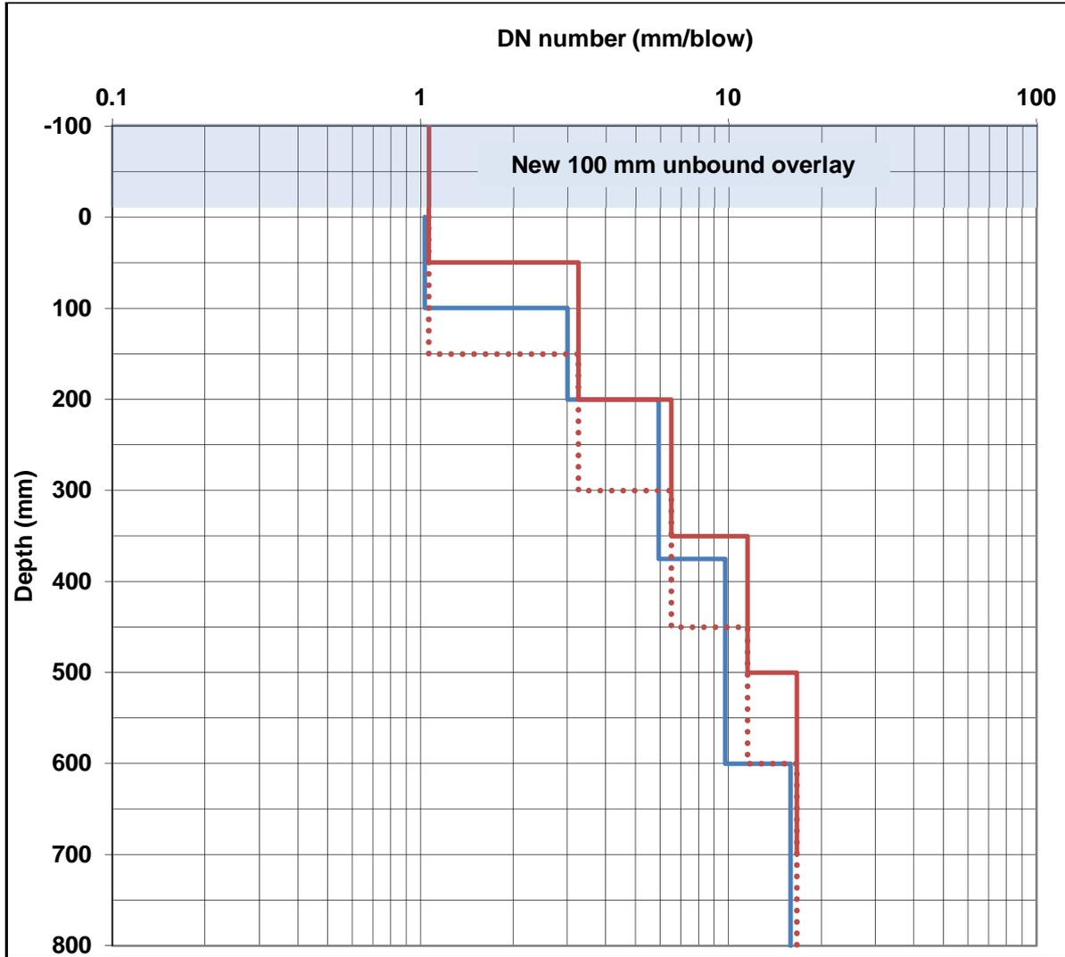
Figure A5. Rehabilitation alternative: 100 mm unbound granular overlay
