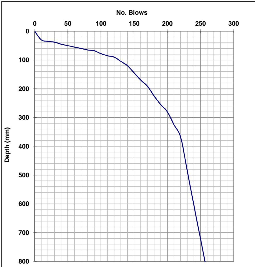
Figure 1. Typical DCP curve
