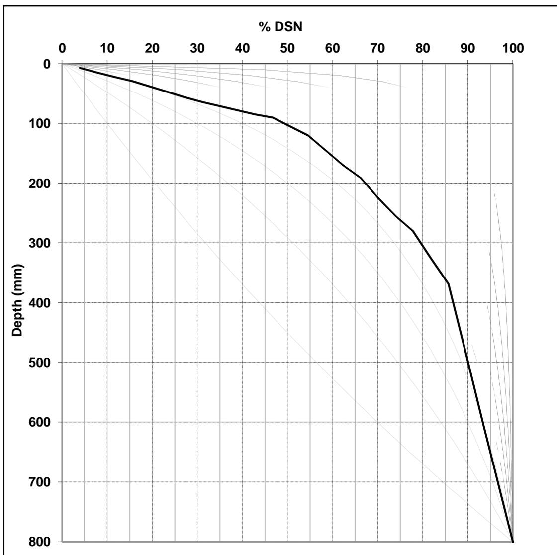
Figure 5. Typical balance curve of a well balanced shallow pavement (BN<sub>100</sub> = 50)
