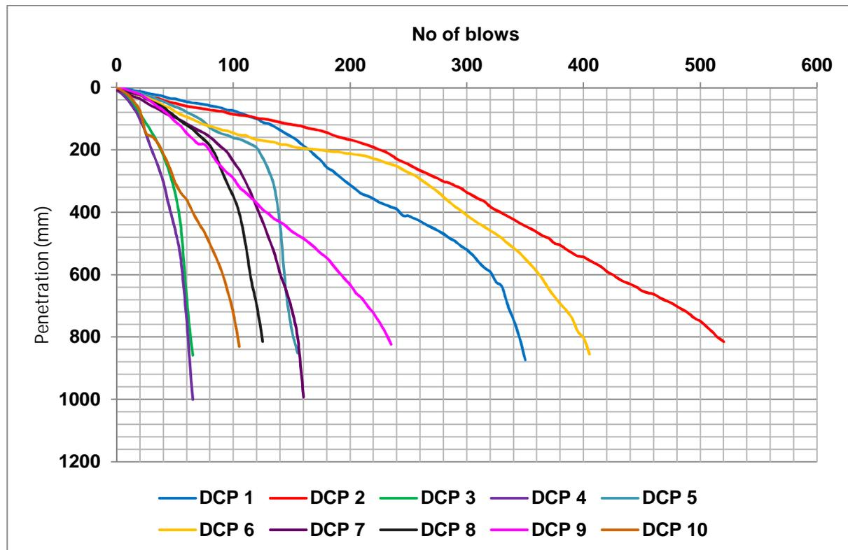
Figure 8 Layer Thickness Estimated from DCP Penetration Rate
