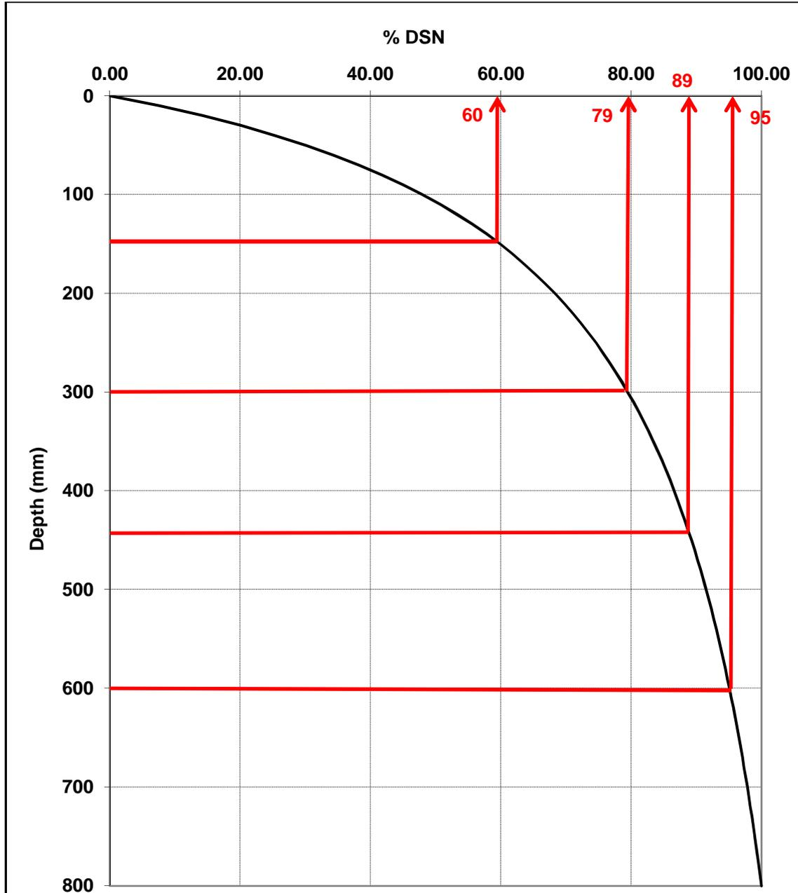
Figure A3. Determine required pavement layer properties from Balance curve.
