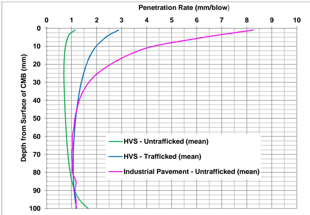
Figure 9. Comparison of DCP penetration rate of upper 100 mm between Industrial pavement and HVS test pavements.
