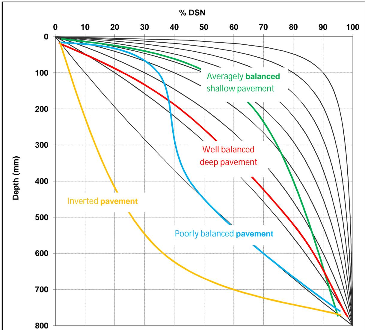
Figure 4. Typical pavement types classified in terms of pavement strength-balance
