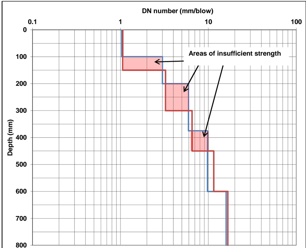
Figure A4. Existing and required layer strength diagrams
