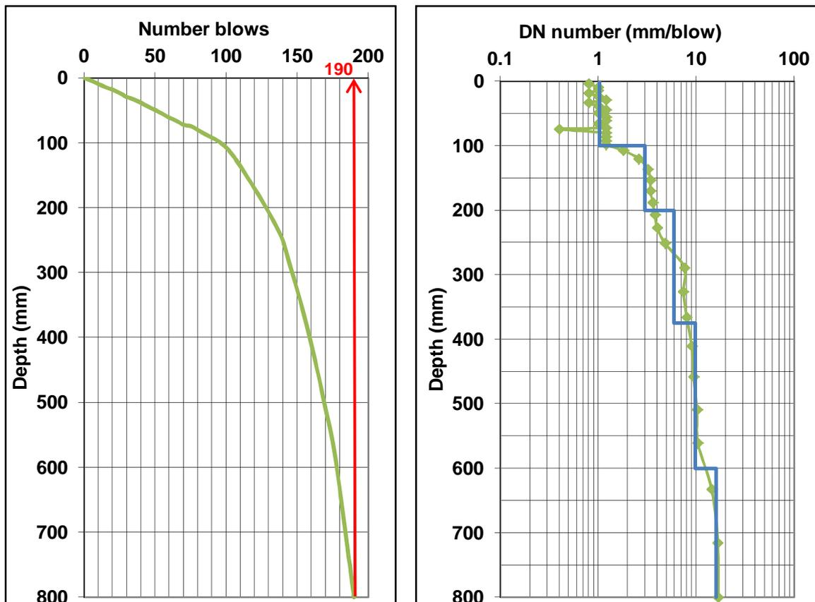
Figure A1. DCP curve and layer strength diagram for measured DCP data
