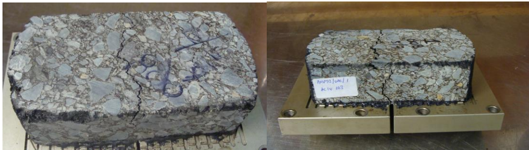
Figure 4 Test Specimens failed
