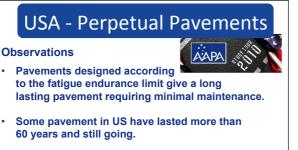
The Fatigue Endurance Limit is an accepted concept for pavement design in the US.
