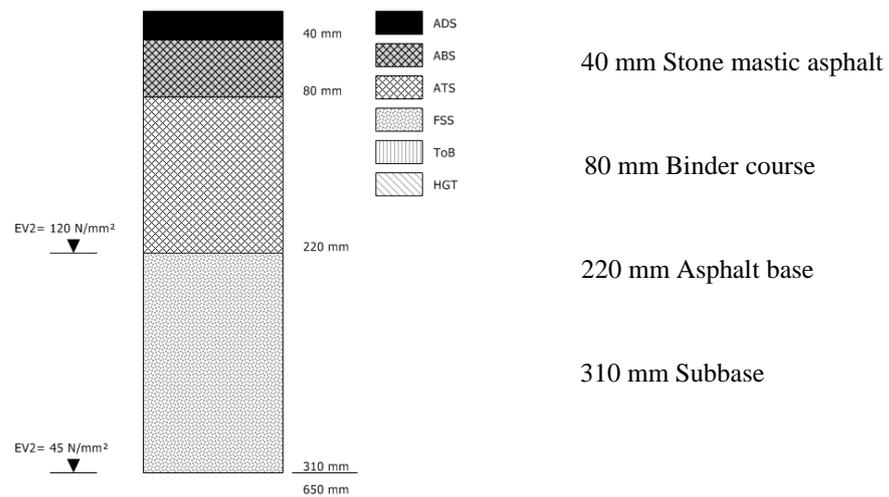
**Figure 8: Layer structure of the chosen pavement**
