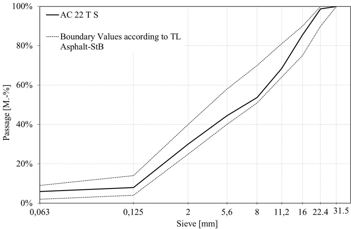
**Figure 1: Grading chart for the three asphalt base variations AC 22 T S**
