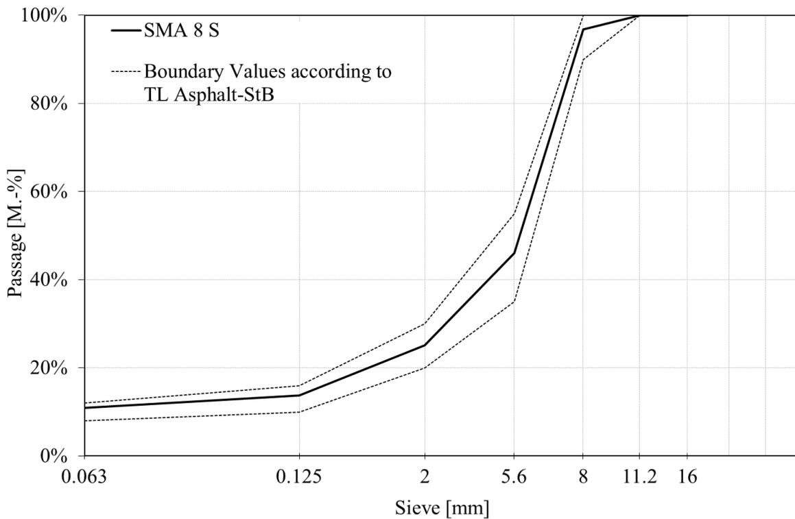
**Figure 2: Grading chart for the eight asphalt surface course variations SMA 8 S**
