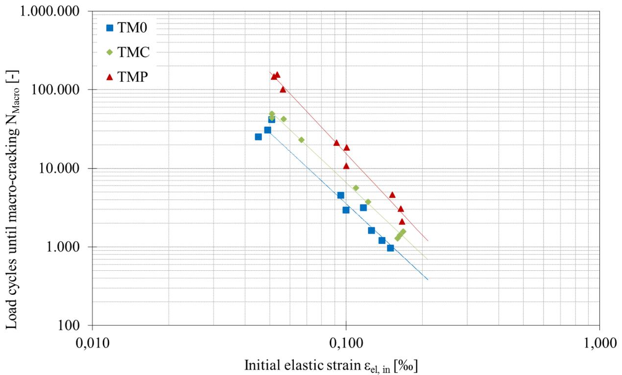
**Figure 3: Fatigue of the three asphalt base variations**
