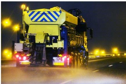
**Figure: 1 Sprinkling de-icing materials**
