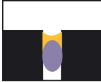
Figure 5. Backer Rod (shown as an ellipse) as a Bond Breaker [31]
