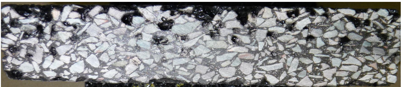
Figure 3: Typical distribution of voids in a PMA layer (cut of core specimen)
