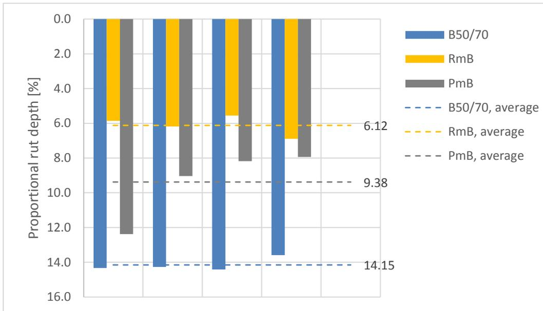
Figure 7: Wheel-tracking test results (proportional rut depth)
