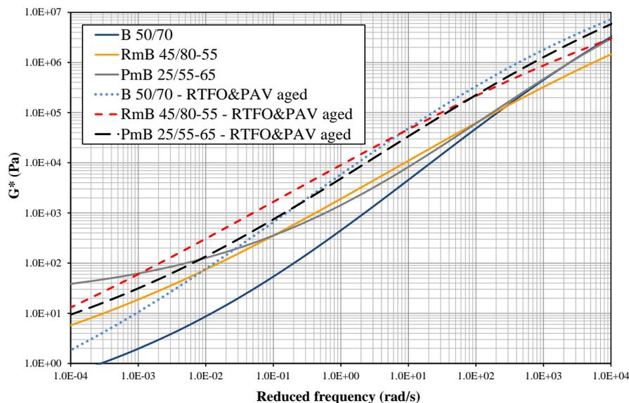
**Figure 1: Master curves of different binders at 60 °C**
