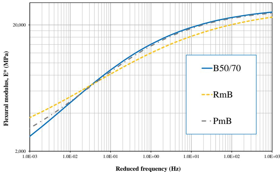
Figure 9: Dynamic modulus master curves of the asphalt mix with different binders
