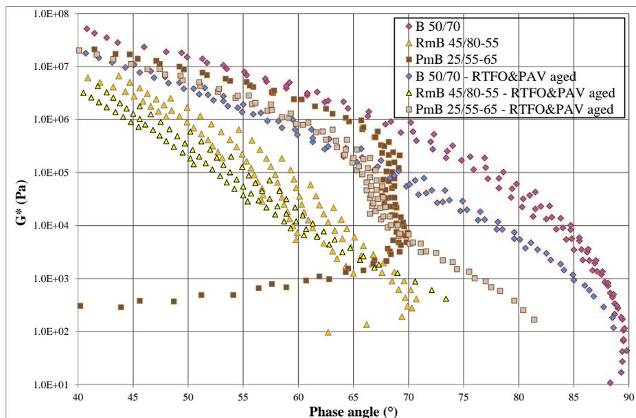
**Figure 2: Black diagram of the different binders**
