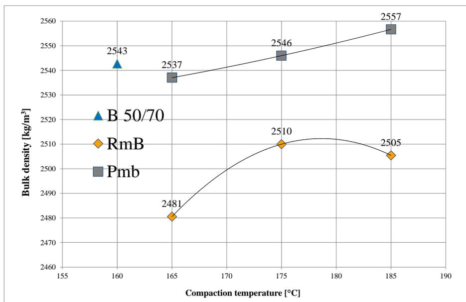
Figure 4: Determination of the laboratory compaction temperatures by using the equi-viscous method
