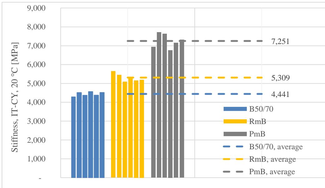
**Figure 6: IT-CY stiffness test results at 20 °C**
