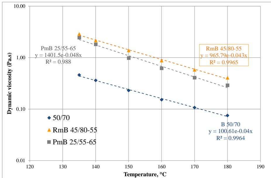
Figure 3: Dynamic viscosity test results
