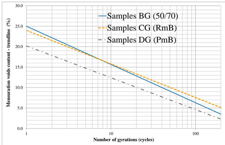
**Figure 5: Workability test results of the asphalt mix with different binders**
