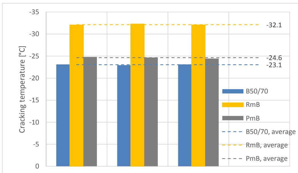
Figure 8: Low-temperature cracking test results
