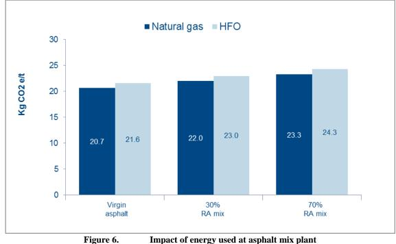
The CO<sub>2</sub> emissions from utilities were comparable for the three asphalt mixes. As expected, CO<sub>2</sub> emissions were slightly higher for the mixes containing RA, reflecting the higher processing temperatures and energy required due to the moisture in the RA. The use of HFO as the energy source instead of natural gas yielded only marginally higher emissions of around 1 kg CO<sub>2</sub> e/t.
