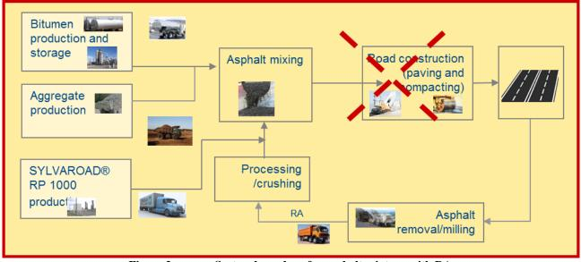
Figure 2. System boundary for asphalt mixture with RA
