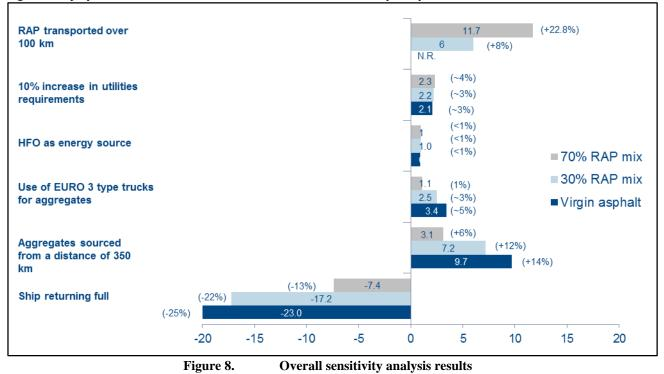
The transportation of raw materials had by far the greatest impact on emissions. The key element was the distance between the asphalt plant and the raw material source. In the case of RA, the milling location needs to be taken into consideration. The type of the truck used for transportation had a more limited impact on the emissions, and the utilities in general are minor contributors.
