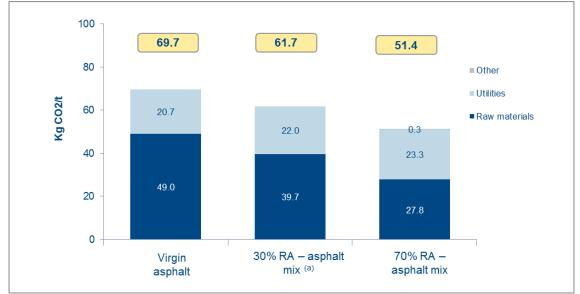
Figure 3. Carbon footprint of the different asphalt mixes based on "locally" sourced aggregates
