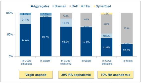
Figure 4. Breakdown of materials' contribution to carbon footprint
