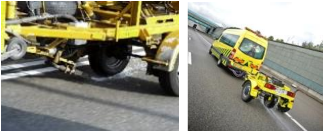
Figure 1: Example of a skid measuring device (RAW 72) for measuring wet skid resistance in the longitudinal direction as is in use in the Netherlands
