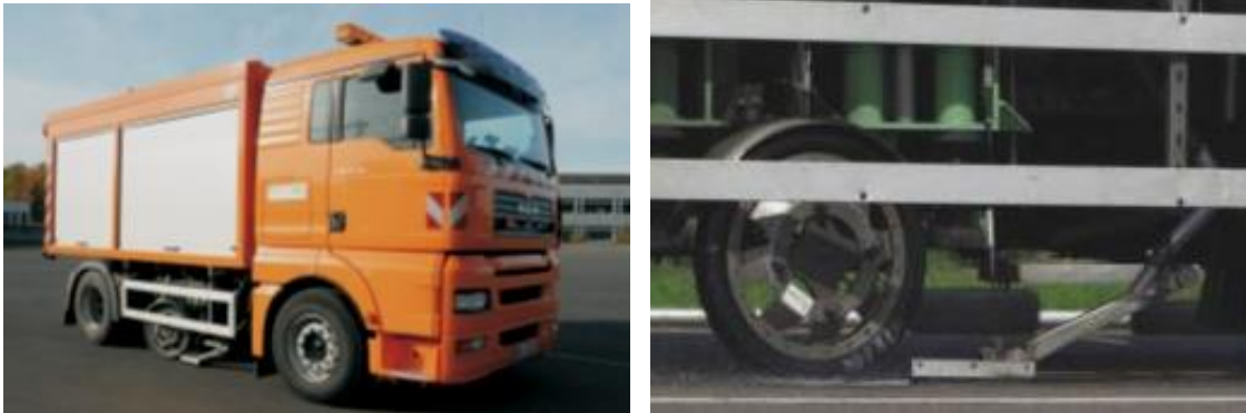
Figure 3: Example of a Sideway Force device (SKM) for measuring skid resistance in the transversal direction
