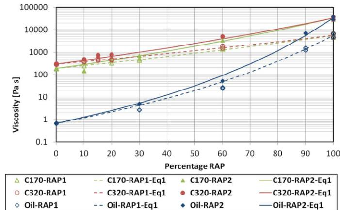
Figure 3: Complex viscosity as measured in the DSR at 1 rad/s and 60 °C
