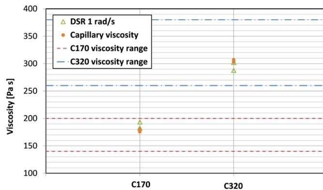
**Figure 2: Comparison of viscosity readings from the DSR and capillary viscometer**
