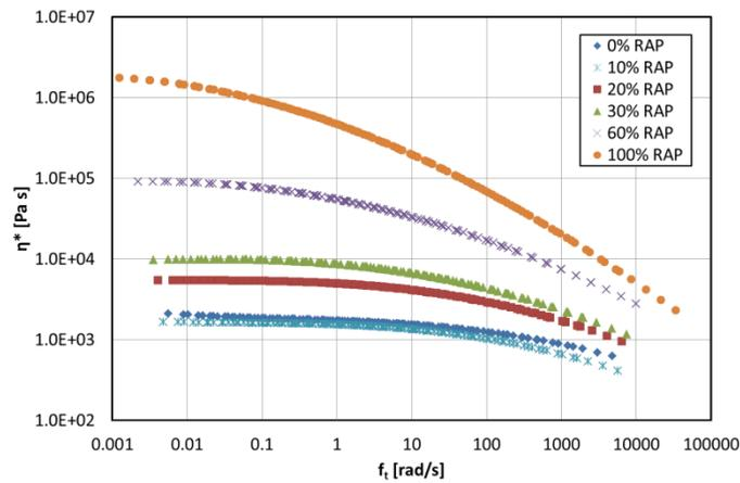
**Figure 1:  $\eta^*$  master curves at 45 °C reference temperature for C320 and RAP1**
