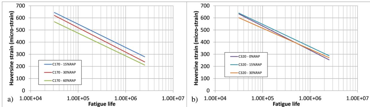
Figure 5: Median fatigue curves
