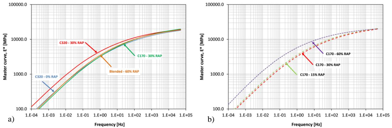
Figure 4: Flexural modulus master curves
